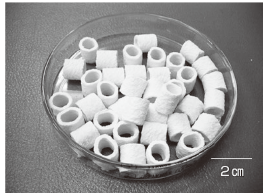
Fig. 1-3 Plastic filter used for the closed recirculating culture system.
